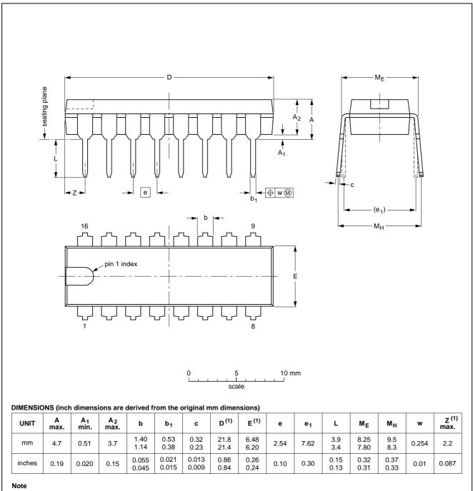
1. Plastic or metal protrusions of 0.25 mm maximum per side are not included.
